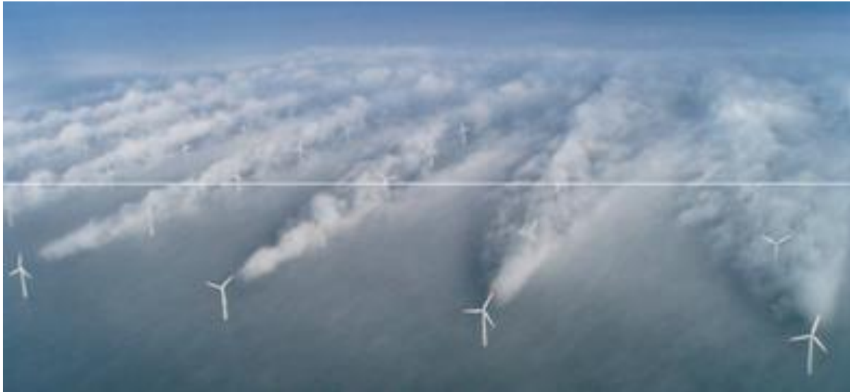
Plate 17: Illustration of the wind farm wake effect.
